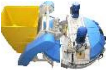
To best meet your needs, the feed side comes with either a closed cover (for you to fit your own chute), open top, optional integrated skip hoist or a built-in aggregate loading hopper.
